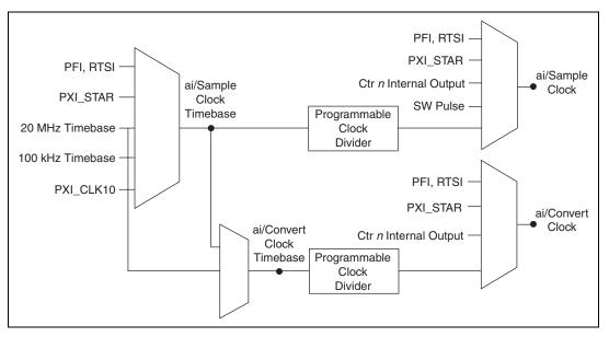
Figure 4-7. Analog Input Timing Options
